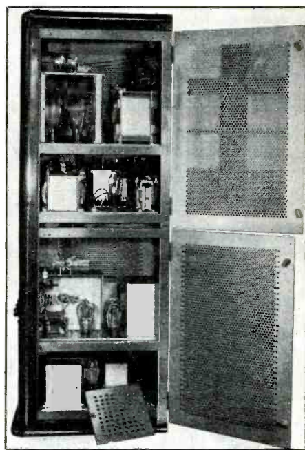
The RCA 100 watt VHF transmitter used for the W9XZK operations ran AM mode from the tower in Chicago's Field Building.
